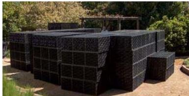
*This modular rainwater cistern was placed underground to collect runoff from impervious surfaces for reuse as landscaping irrigation at a private residence in Palo Alto.*
